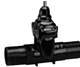
Series 46/64 Gate valve with short spigot ends DN50-300 PN16 GP240GH External epoxy coating
