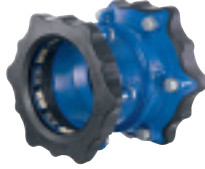
Series 631/00 Supa Maxi™ universal tensile straight coupling DN50-600 PN16 Ductile iron
