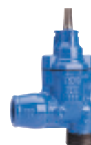
Series 11/30 Service connection angle valve with external thread on inlet and tensile socket end for PE pipes on outlet DN25-50 PN16 Ductile iron
