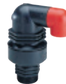
Series 701/40 Combination air valve DN20, 25 and 50 Threaded BSP 3/4", 1" or 2" PN16 Reinforced polyamide
