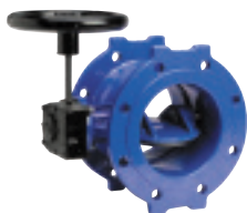
Series 756/100 Butterfly valve Double eccentric Double flanged Integral seat IP 67 gearbox DN200-2800 PN10/16 Ductile iron
