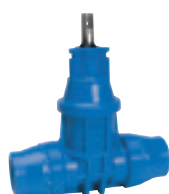
Series 16/50 Service connection valve with tensile socket ends for PE pipes DN25-50 PN16 POM (Polyoxymethylene)
