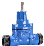
Series 03/90 Service connection valve with PRK couplings for PE pipes DN20-50 PN16 Ductile iron
