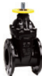
Series 15/78 Flanged gate valve with ISO top flange DN50-400 PN10/16 Ductile iron External PUR coating
