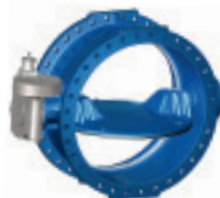
Series 756/102 Butterfly valve Double eccentric Double flanged Stainless steel seat ISO-input gearbox DN200-2800 PN10/16 Ductile iron
